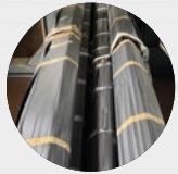
The bars are double packed in semiflex (thick black plastic packaging) to protect them from humidity.
